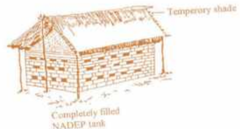
Filling of NADEP Compost tank
